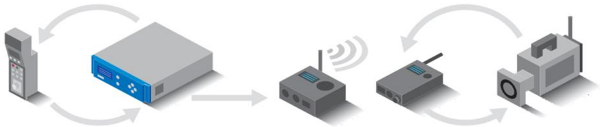
Fig 1. A simple Uni-directional camera control setup
