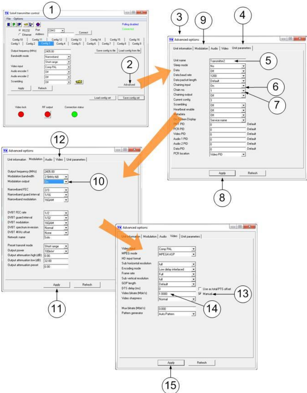
Figure 12-9 – Configuring Transmitter 2 for Chaining with Manual Bit Rate
