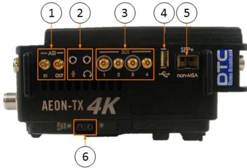
Figure 3-3 AEON-TX Right Panel
